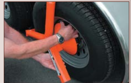
3. Slide the hooks over the wheel and insert the wheel nut cover.
