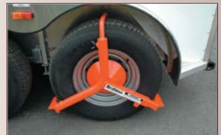
4. Insert the telescoping hook and snap the lock into the nearest hole.
